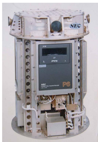
Fig. 12. Artificial snow crystal growth experiment under zero-gravity in Space Shuttle Callenger. (NASA, USA, NEC and KELK, Japan, 1983)
