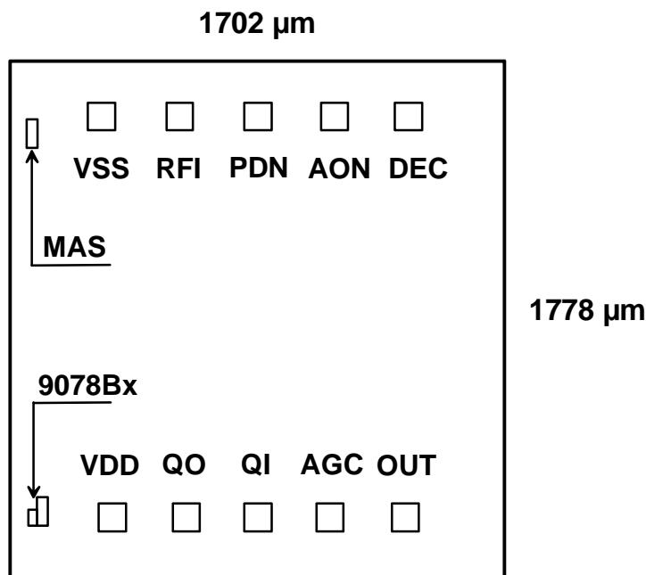
DIE size = 1.70 x 1.78 mm; PAD size = 100 x 100 μm
